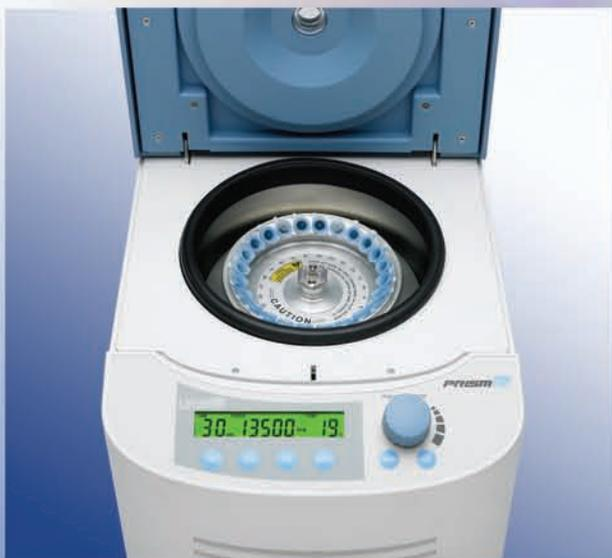
The *Prism's* uniquely designed 24-place rotor allows easy access to the tops of sample tubes, allowing for faster work flow. The individual tube slots in the solid rotor support tubes along their length to eliminate tube deformation or cracking even at the highest speed settings. In the event of a tube failure, tube pieces and samples are contained within the sample well.
